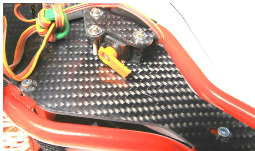
The arm should be pointing up when being in the high position thus allowing your Drop Pod to be locked and secured when flying.
