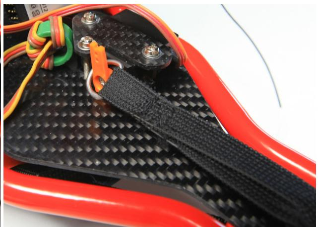
You will simply need to operate your switch to drop the parachute. Indeed, the servomotor's arm will let the Drop Pod open when moving down close to the plate, thus letting the parachute open by itself thanks to the system inertia.
