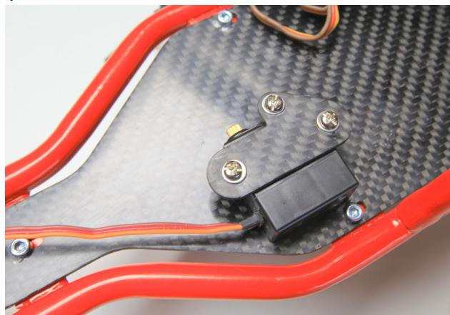
The servomotor won't move at all thanks to this holding system.
