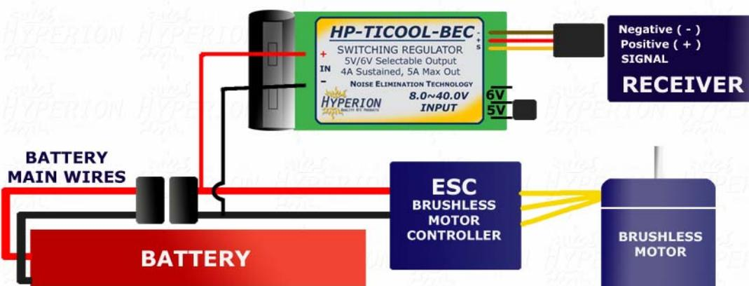
This option is recommended for models which do not use a balance connector (for example, if using NIMH packs) or models which use more than one lithium pack to power the model, connected in series or in parallel.
