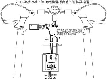
Assemble Folding Landing Gear as this illustration. 將折合腳架座如圖組裝。
