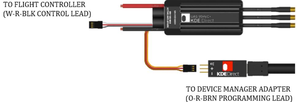
Pay close attention to proper wiring as shown in the diagrams. The ESC is automatically powered via the USB DMA when using the Programming Lead (orange-red-brown cable). External power is NOT required to properly arm and program the microcontroller in most cases.
