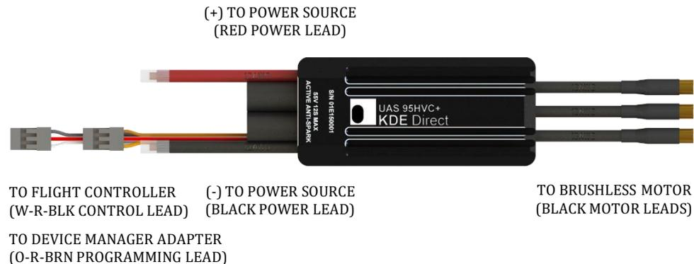
Pay close attention to proper wiring as shown in the diagram above. Ensure the polarity is correct and proper soldering techniques are used when connecting the power source and-brushless-motor-to prevent damaging the ESC.
