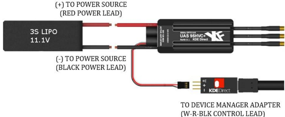
If the ESC does not include the dedicated Programming Lead or does not connect, a 9V to 12V power source (2S or 3S LiPo preferred, 25V maximum) is required for powering the ESC during programming. Once external power is properly applied to the ESC, the microcontroller is programmed via connection of the DMA to the Control Lead (white-red-black cable).
