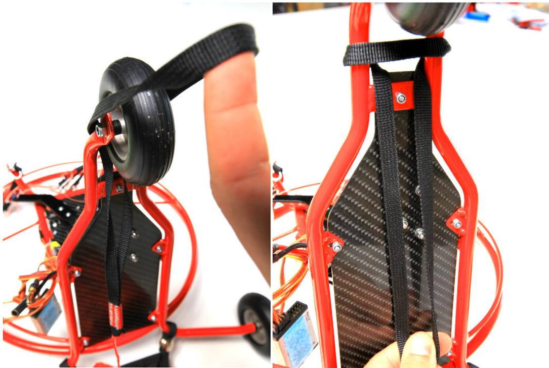
Then, connect the small servomotors that will be used to release the Rescue 1.8 to your receiver. Assign an easily accessible switch on your radio control (rather a 2-position switch). Put the servomotor in the release position, and then attach the arm parallel to the carbon plate. Screw everything together.
