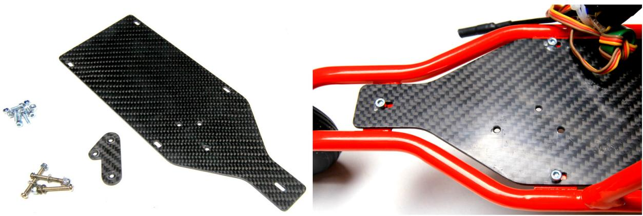
Now you can put the servomotor on. For this, you need the carbon fiber - servomotor holding - plate and the 3-20 M3 screws with washers and nuts.
