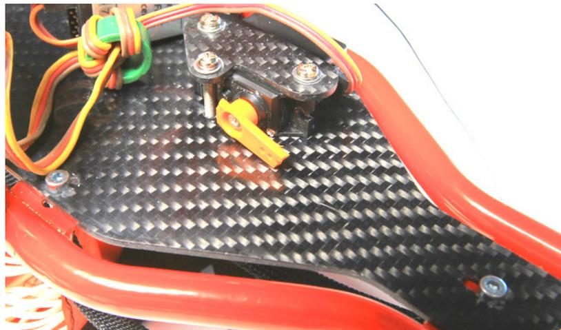
The arm should be pointing up when being in the high position thus allowing your Drop Pod to be locked and secured when flying.
