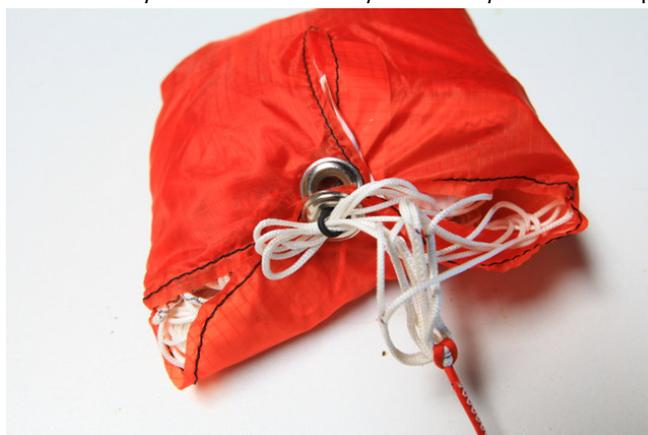
Please often check that the container is well closed and kind of locked thanks to the lines. Do not hesitate to ventilate and unfold your parachute if it is stored wet.
