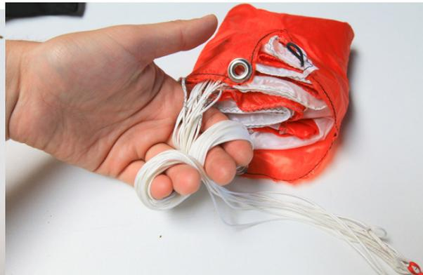
Grab the lines and wind them round your fingers till it looks like an 8 in order to store the lines in the container. Then house the lines inside the container just in front of the parachute's trailing edge.
