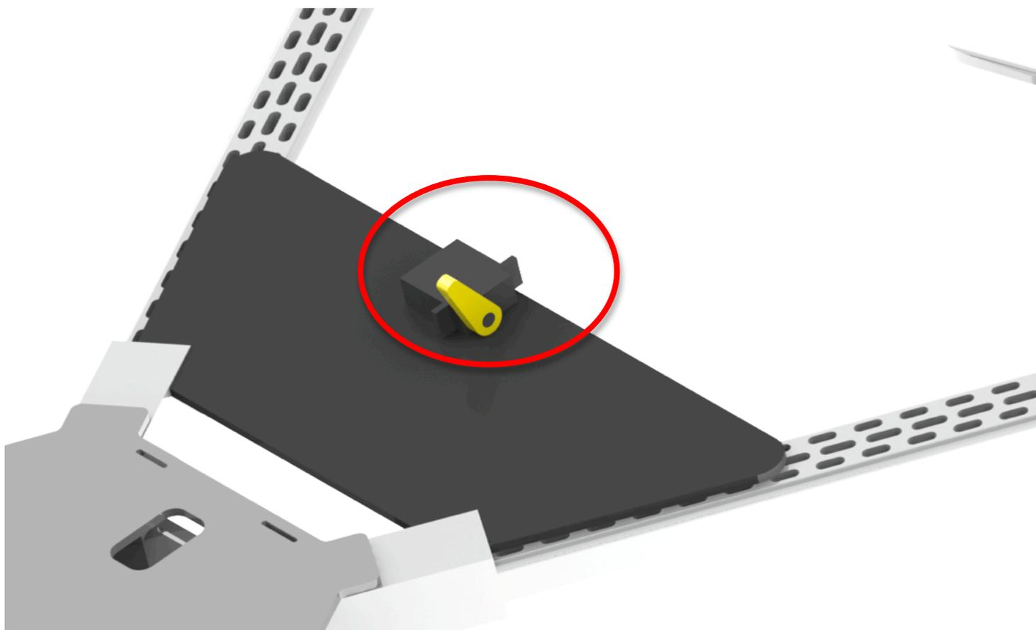
The locked position of the actuator corresponds to a vertical rudder. The open position corresponding to a horizontal lifting beam, directed towards the rear.
