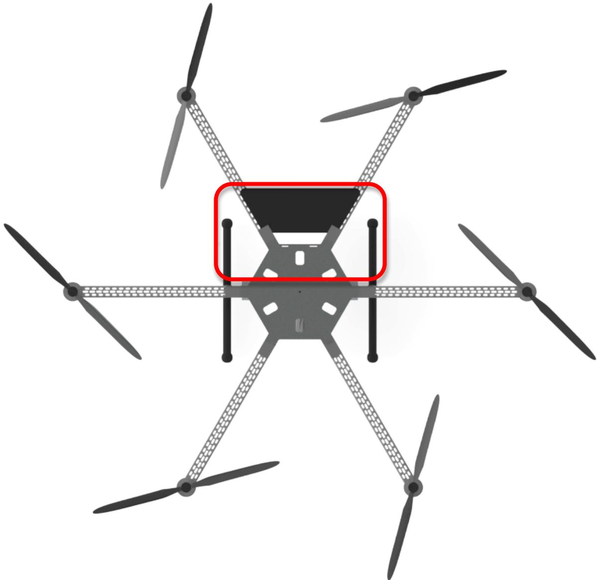
To achieve this plate trapezoidal, you can use PVC, or a plate of glass fiber mixed with epoxy.
