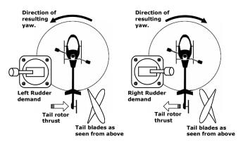
When performing the final checks of the gyro installation, you should also check the correct operation of the gyro direction. To do this set the gyro in AVCS mode (LED on) and rotate the helicopter at least 90 degrees counter-clockwise. In an attempt to oppose the rotation and maintain the aircrafts heading the gyro should have now moved the tail blades in the same manner as if right rudder was applied. If this test fails you should check the reversing of your radio and reconfigure the gyro.
